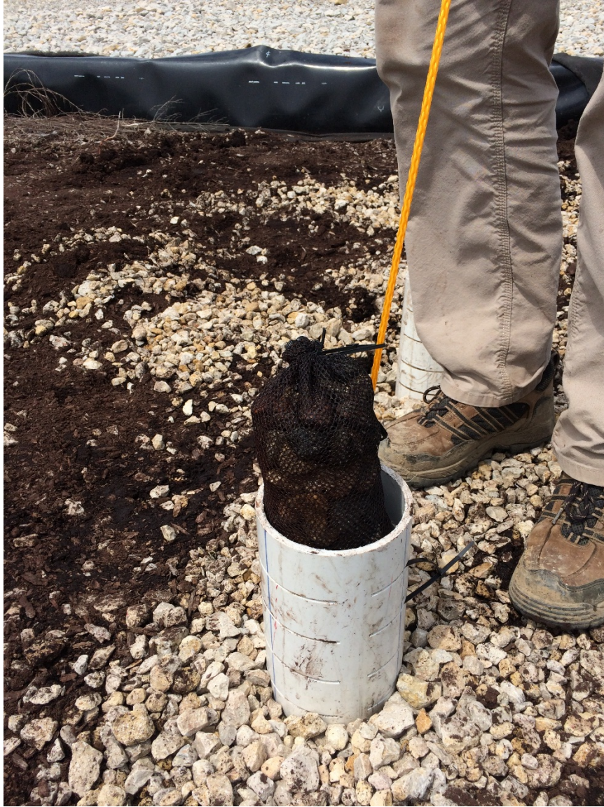
Figure B.4 Mesh bag containing sterile rocks deployed in the SAGR for biofilm sampling.
